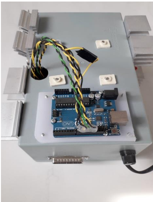
Fig. 9. Power supply & controller
