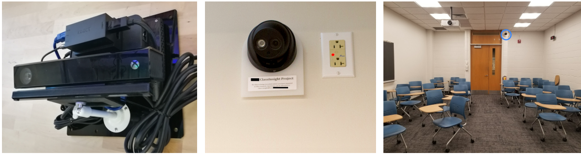
Fig. 2. Left: Early version of EduSense, using a Microsoft Kinect One depth camera and Intel NUC. Center: Current system, which uses networked 4K cameras that are accessed from a central server ( partially anonymized for review ). Right: example classroom from our deployment with instructor-facing camera circled in blue.
