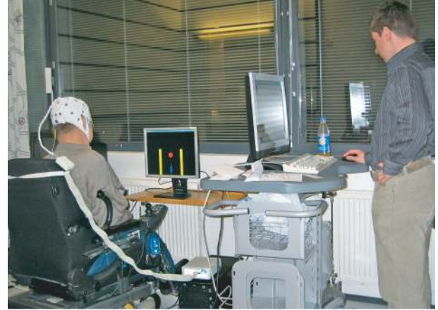
FIGURE 1: A tetraplegic subject using the BCI in his patient room at the rehabilitation centre. The BCI controller is on the subject's right side. The subject's task was to move the red circle to the yellow target on the side of the screen.
