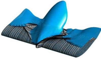
**Figure 8.** Limiting streamlines and recirculation regions shown by isosurface of zero longitudinal velocity (SST  $k-\omega$ , modified airfoil,  $15^\circ$ )
