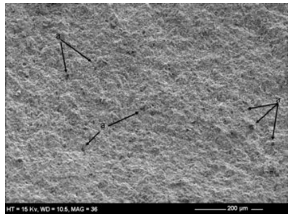
Figure 4 Intact surface of unetched mineral trioxide aggregate after 96 h. An amorphous poorly crystallized superficial gel structure and the cross-section of several microchannels (a) can be seen (original magnification: 36×).
