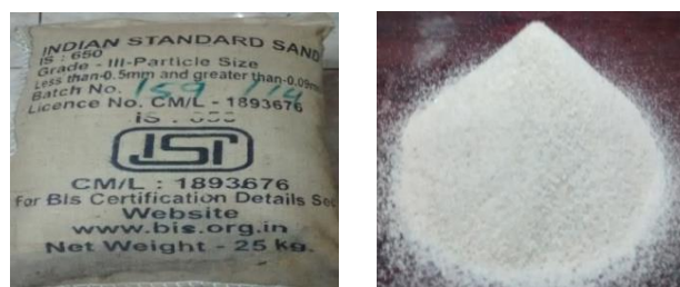
Figure 5. Grade-III: Less than 0.5 mm greater than 0.09 mm.
