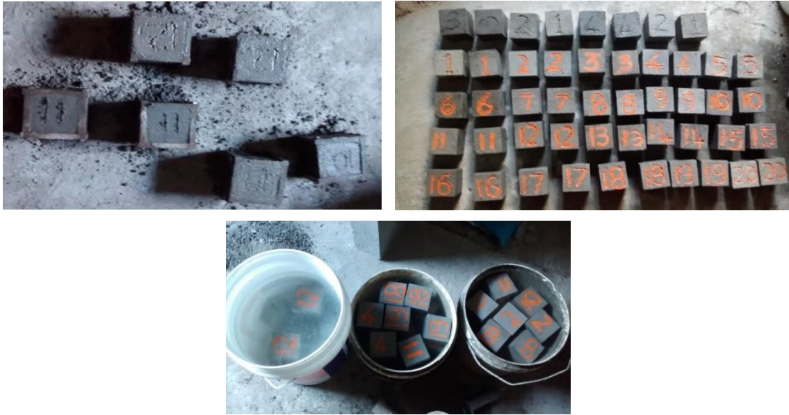
Figure 8. Casting and curing of specimens.
