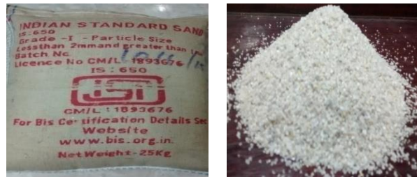
Figure 3. Grade-I: Less than 2 mm greater than 1 mm.
