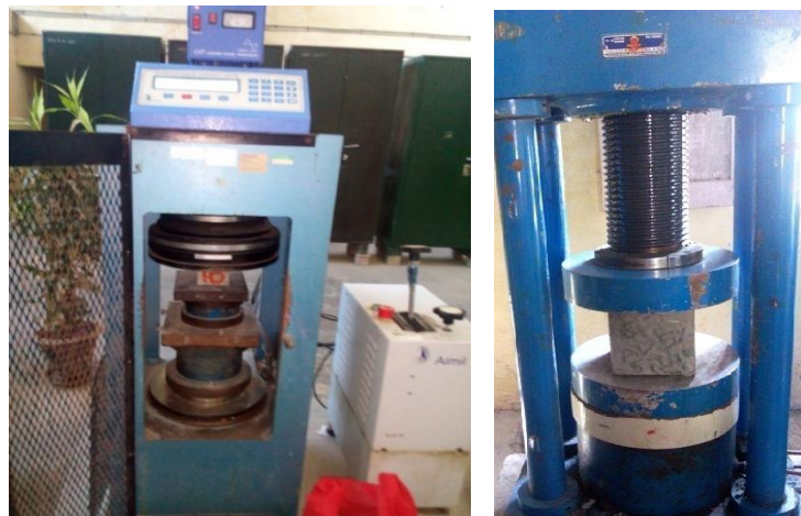
Figure 9. Mortar cube compressive strength test.
