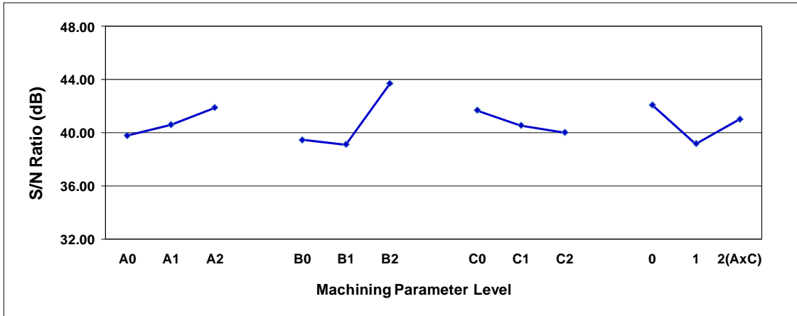
Figure 4: Response graphs of mean and S/N ratio for circularity
