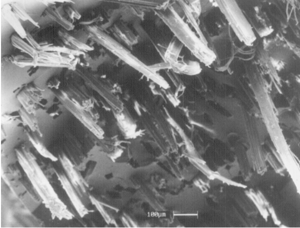
Figure 9. Fibre pull out and breakage in composites reinforced with 23 wt% untreated jute fibres.
