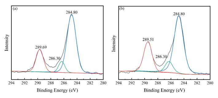
**Figure 6.** C1s XPS spectra of malachite surfaces as follows: (a) treated with Na<sub>2</sub>S, (b) treated with  $(NH_4)_2S$ , Na<sub>2</sub>S = 6 × 10<sup>-2</sup> mol/L,  $(NH_4)_2S$  = 6 × 10<sup>-2</sup> mol/L.
