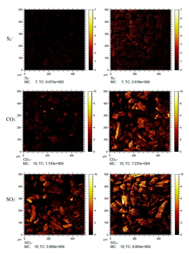
**Figure 11.** ToF–SIMS negative ion images of the malachite surface as follows: (**a**) treated with Na<sub>2</sub>S, and (**b**) treated with  $(NH_4)_2S$ , Na<sub>2</sub>S = 6 × 10<sup>-2</sup> mol/L,  $(NH_4)_2S = 6 \times 10^{-2}$  mol/L.
