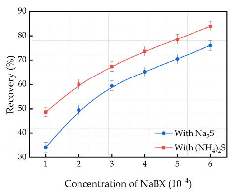
**Figure 2.** Flotation recovery of sulfidized malachite with  $(NH_4)_2S$  and  $Na_2S$  as a function of NaBX concentrations:  $Na_2S = 6 \times 10^{-2} \text{ mol}/\text{L}$ ;  $(NH_4)_2S = 6 \times 10^{-2} \text{ mol}/\text{L}$ ;  $NaBX = 2 \times 10^{-4} \text{ M}$ ;  $pH = 8.7 \pm 0.05$ .
