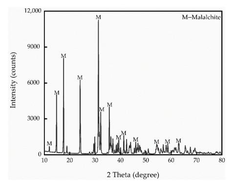
Figure 1. X-ray diffraction of malachite sample.
