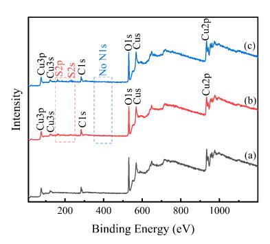
**Figure 10.** XPS survey spectra as follows: (a) pure malachite, (b) treated with Na<sub>2</sub>S and (c) treated with (NH<sub>4</sub>)<sub>2</sub>S, Na<sub>2</sub>S =  $6 \times 10^{-2}$  mol/L, (NH<sub>4</sub>)<sub>2</sub>S =  $6 \times 10^{-2}$  mol/L.
