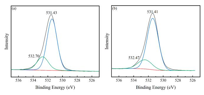
**Figure 7.** O1s XPS spectra of malachite surfaces as follows: (**a**) treated with Na<sub>2</sub>S, (**b**) treated with  $(NH_4)_2S$ , Na<sub>2</sub>S = 6 × 10<sup>-2</sup> mol/L,  $(NH_4)_2S = 6 \times 10^{-2}$  mol/L.
