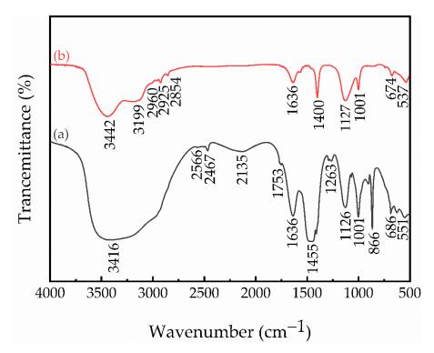
Figure 4. FTIR spectra of (a) sodium sulfide and (b) ammonium sulfide.
