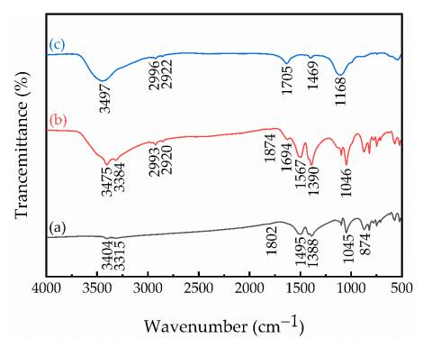
**Figure 5.** FTIR spectra as follows: (a) pure malachite, (b) malachite + Na<sub>2</sub>S and (c) malachite +  $(NH_4)_2S$ , Na<sub>2</sub>S = 6 × 10<sup>-2</sup> mol/L,  $(NH_4)_2S$  = 6 × 10<sup>-2</sup> mol/L.
