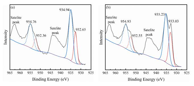
**Figure 9.** Cu 2p XPS spectra of malachite surfaces as follows: (a) treated with Na<sub>2</sub>S, (b) treated with  $(NH_4)_2S$ , Na<sub>2</sub>S = 6 × 10<sup>-2</sup> mol/L,  $(NH_4)_2S$  = 6 × 10<sup>-2</sup> mol/L.
