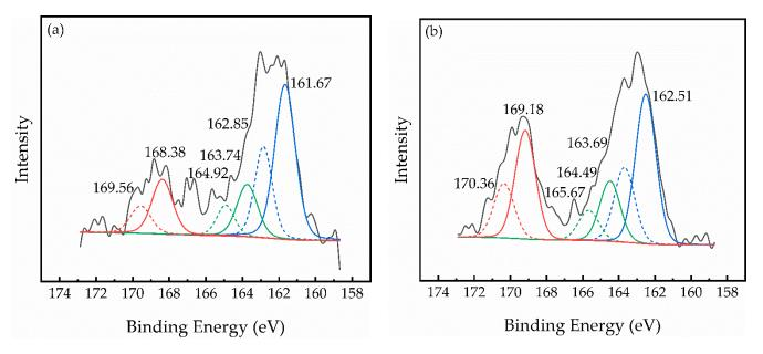
**Figure 8.** S 2p XPS spectra of malachite surfaces as follows: (**a**) treated with Na<sub>2</sub>S, (**b**) treated with (NH<sub>4</sub>)<sub>2</sub>S, Na<sub>2</sub>S =  $6 \times 10^{-2}$  mol/L, (NH<sub>4</sub>)<sub>2</sub>S =  $6 \times 10^{-2}$  mol/L.
