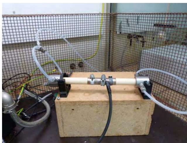
Figure 1. Top: schematic diagram of the cylindrical DBD reactor, with 1 = inner electrode, 2 = discharge gap, 3 = dielectric tube, 4 = outer electrode; Bottom: picture of the DBD reactor.
