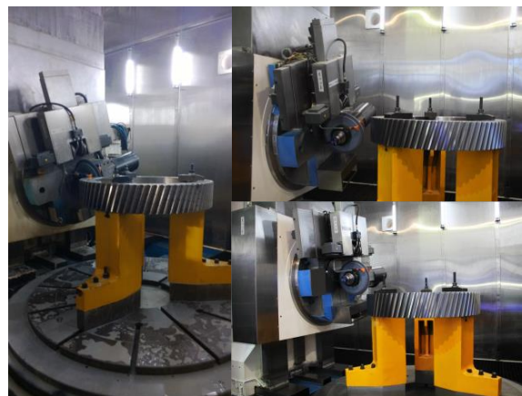
Figure 16. The grinding process of the SKMC-1200W/08 gear profile grinding machine.
