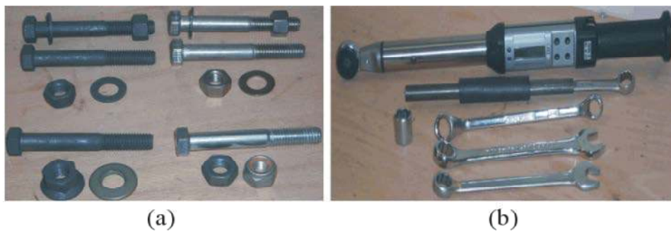
Fig. 2: (a) Bolts, Nuts and washers used during tests, (b) Torque Wrenches used
