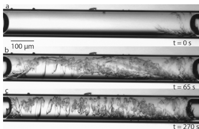
Figure 4. Crystallization of 1 mol/kg sodium sulfate solution mixed with 0.051 mol/kg borax in a glass capillary at the start (a) and after 65 s (b) and 270 s (c). Both phase III and phase V anhydrous crystals form simultaneously (a). At the end of the shown sequence (c), all needles (phase III) have dissolved. The crystal habit of phase V is altered with respect to that observed in the absence of borax (compare to Figure 3c).
