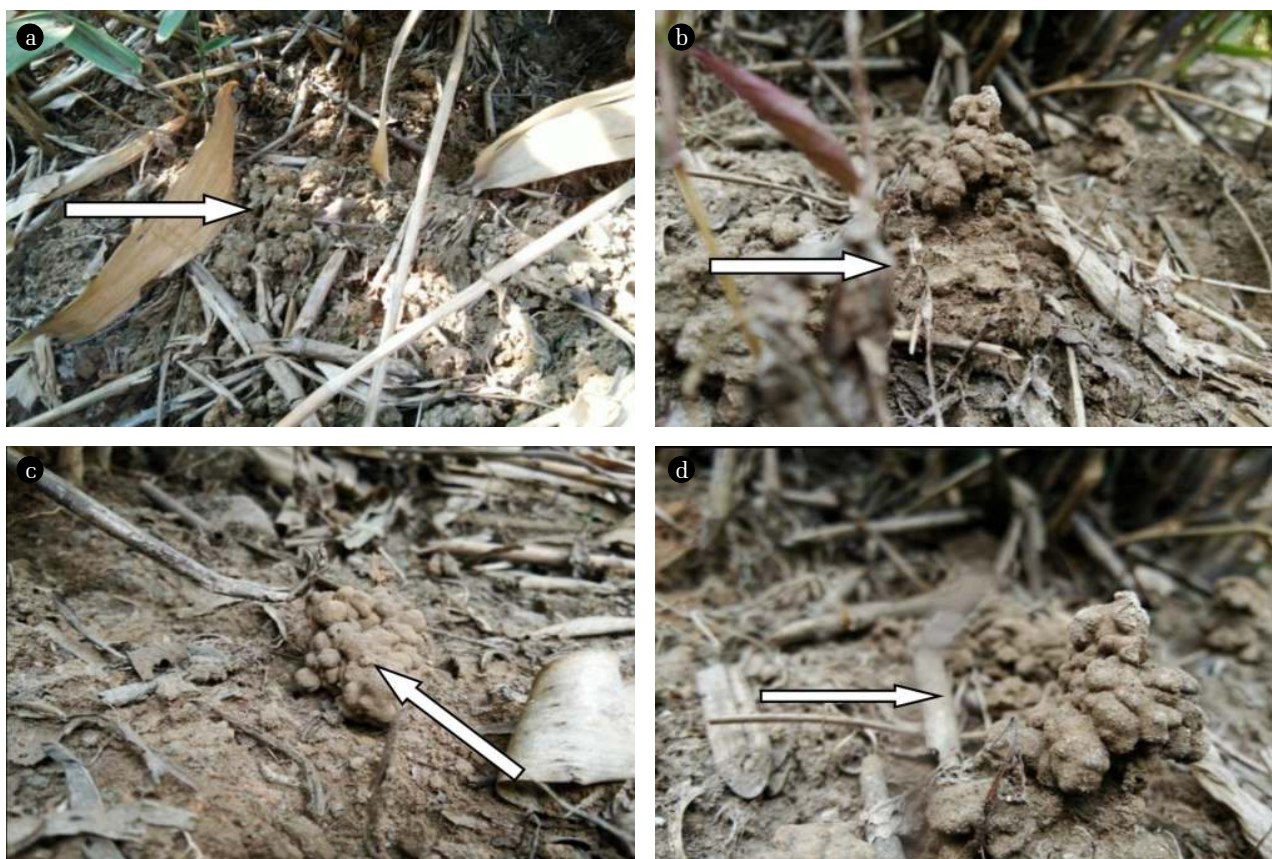
Fig. 3. Photographs showing soil forming hard crust after mixing with cement dust.
