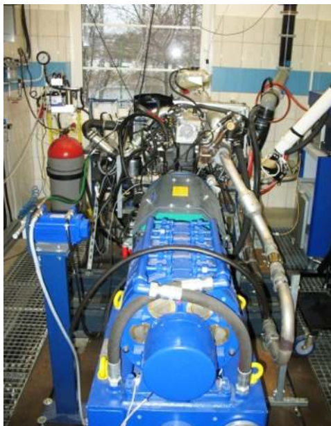
Fig. 2. The test stand with an ADCR engine installed at the engine test stand
