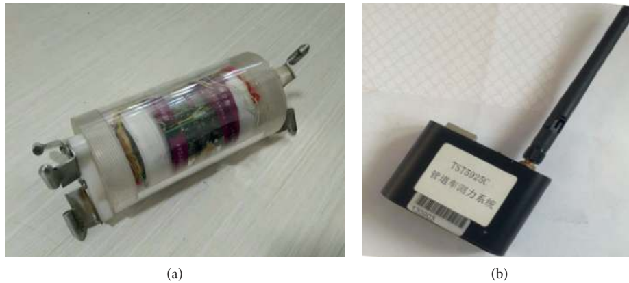
FIGURE 6: The cylinder pipe vehicle force measurement equipment. (a) Force measuring device. (b) Signal receiving equipment.
