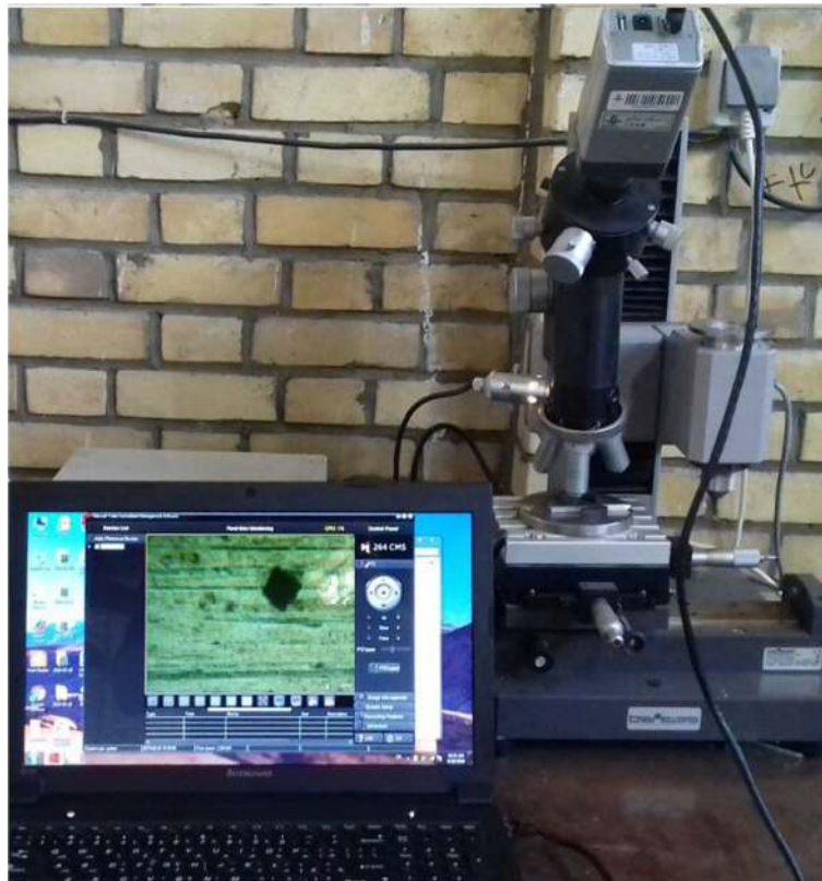
Fig. 9 The used equipment for microhardness testing
