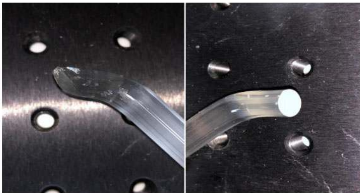
Fig. (2). Shows a damaged tip for (Acteon mini LED) versus a new tip.
