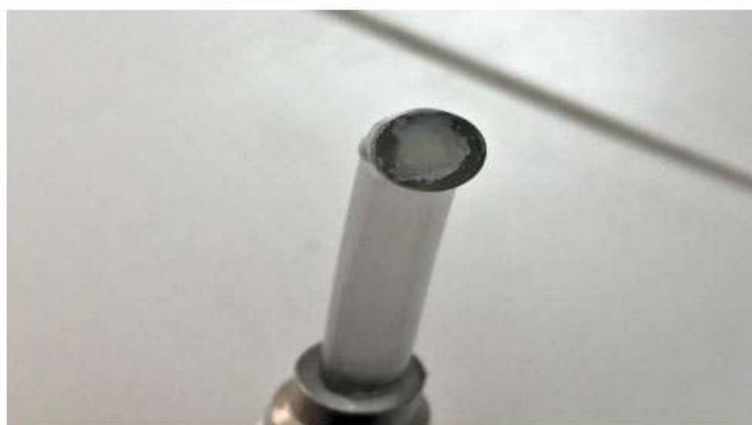
Fig. (1). A layer of composite residue covering most of the tip of one LCU as received before cleaning.
