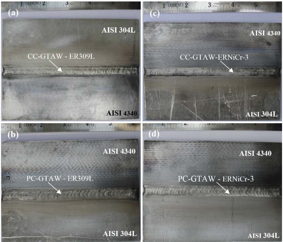
Figure 1. Photographs of the dissimilar weldments of AISI 4340 and AISI 304L employing (a) CCGTAW-ER309L (b) PCGTAW-ER309L (c) CCGTAW-ERNiCr-3 (d) PCGTAW-ERNiCr-3.
