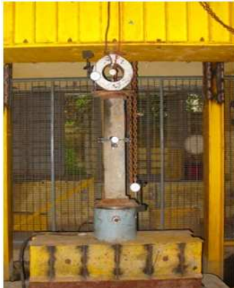
Fig. 3: Column test setup and instrumentation
