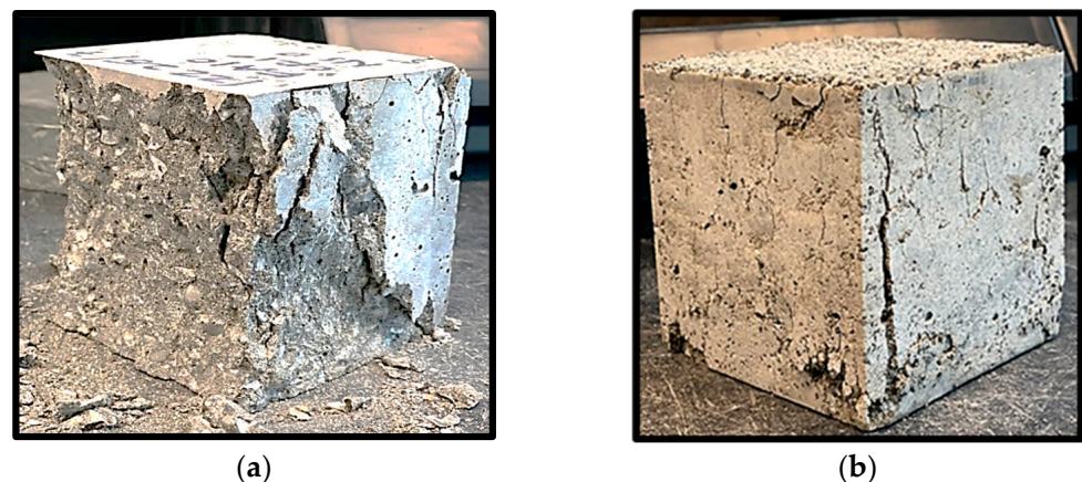
Figure 7. (a) FA40CR0NS4 sample at failure; (b) FA40CR15NS4 sample at failure.
