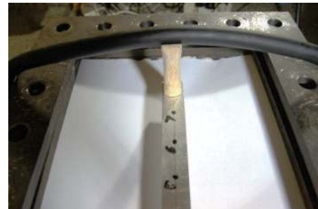
FIGURE 5: Setup diagram of applying the dead load.
