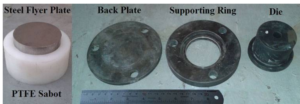
2 Projectile and compaction set-up used in gas gun assisted compacted samples
