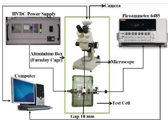
Fig. 1. Complete block diagram of experimental setup under influence of DC electric field with needle plane electrodes [2].
