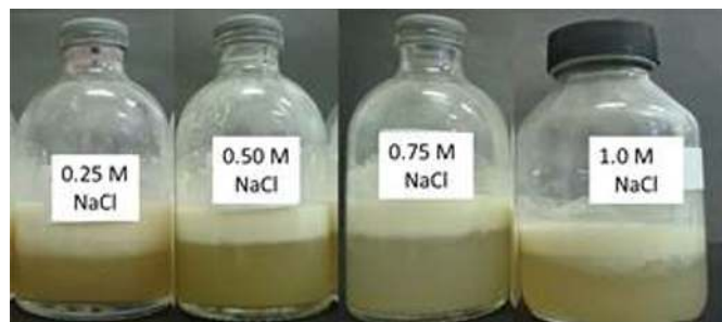
Figure 4. Visual aspect of the lipid-microparticle dispersions, which were produced using tristearin and babacu oil, encapsulated quercetin, and submitted to different ionic strengths under magnetic stirring, after 24 hours of storage under refrigeration.
