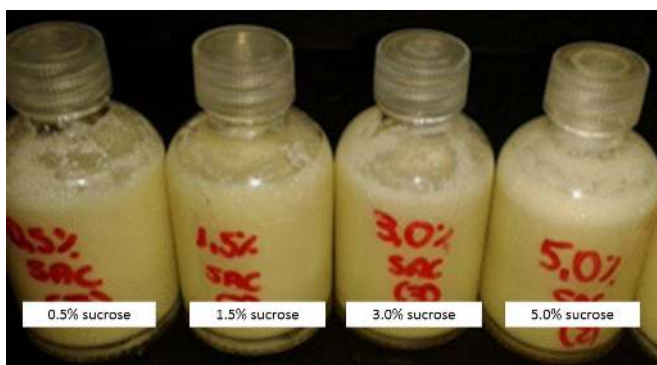
Figure 7. Visual aspect of the lipid-microparticle dispersions, which were produced using tristearin and babacu oil, encapsulated quercetin, and submitted to different sucrose concentrations under magnetic stirring, after 24 hours of storage under refrigeration.
