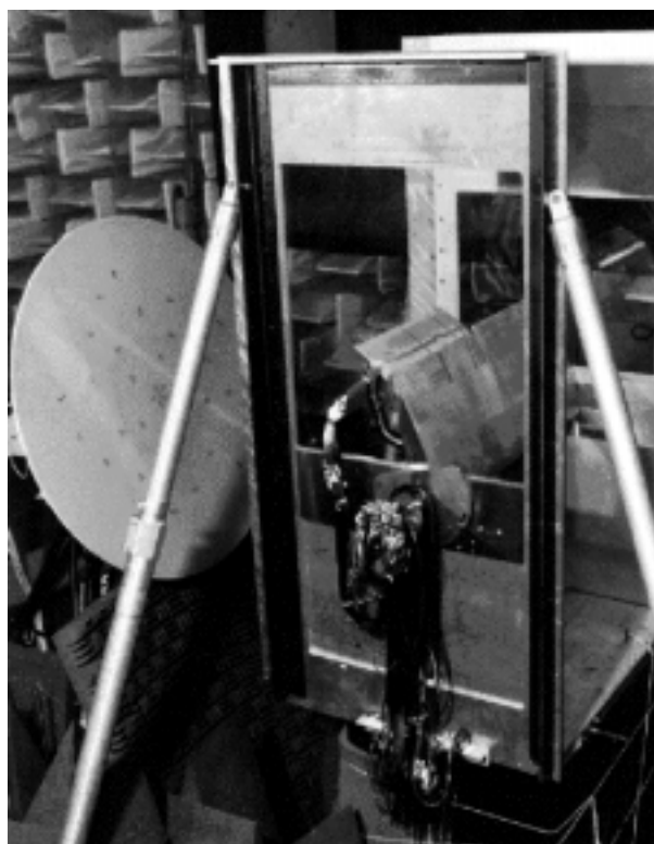
Figure 1. LADA mounted in the QFF on pressure side of model.
