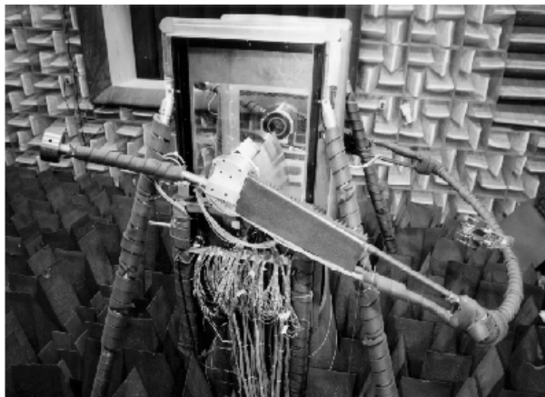
Figure 2. SADA mounted on pivotal boom in the QFF on suction side of model.
