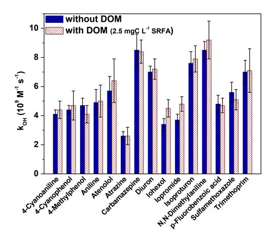
**Figure 4.** Second-order reaction rate constants of hydroxyl radical with fifteen target compounds in the presence and absence of SRFA (2.5 mgC L<sup>-1</sup>) used as reference DOM. Error bars represent 95% confidence intervals of regression lines obtained by competition kinetics experiments.
