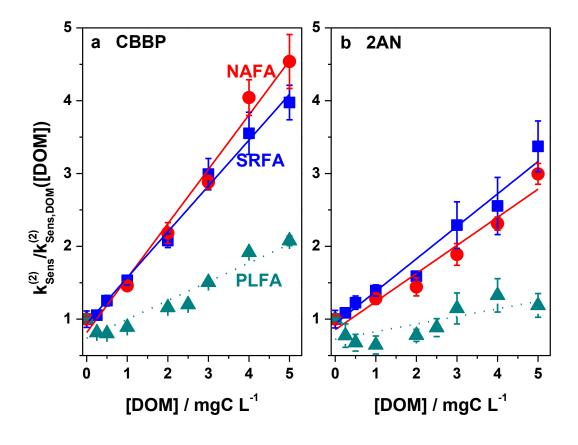
**Figure 3.** Plots of inverse rate constant ratios for sulfamethoxazole (SMX) versus [DOM] and linear regression lines according to eq 6a. Photosensitizers: a) CBBP and b) 2AN. DOMs: ●, Nordic Aquatic fulvic acid (NAFA); ■, Suwannee River fulvic acid (SRFA); ▲, Pony Lake fulvic acid (PLFA).
