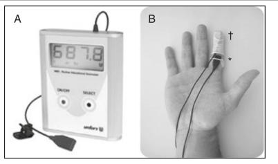
Fig. 2 a The Unfors® NED operational dosimeter. b Positions of the dosimeter sensors: \*P1 (proximal); †P3 (distal)
