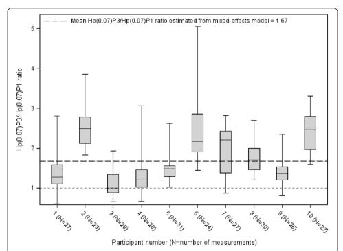
**Fig. 3** Interquartile range box plot of the distribution of the Hp  $(0.07)_{P3}$ /Hp  $(0.07)_{P1}$  ratio (between the radiation dose received by the palm side of the distal phalanx and the proximal phalanx of the index finger) per participant. On the ordinate: the Hp  $(0.07)_{P3}$ /Hp  $(0.07)_{P1}$  ratio in N = 271 paired observations performed in ten study participants. On the *abscissa*: the nominal number of the study participant (the number of repeated measurements per participant)
