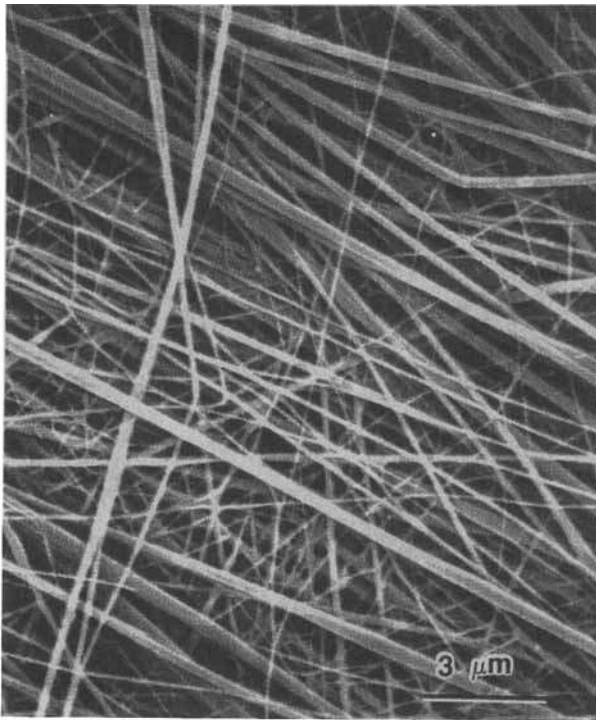
Fig. 2. SEM micrograph of the microfibrils in a drawn sample after extracting the PC matrix.
