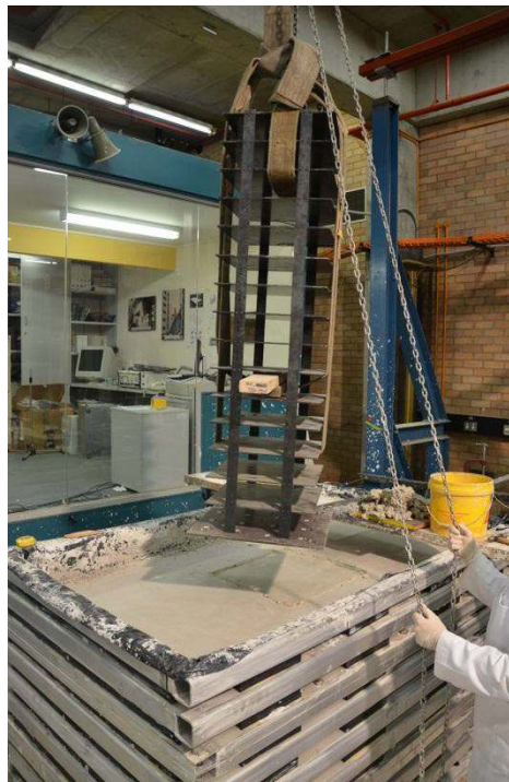
Figure 4.21 Placing the fifteen storey model structure on top of the soil mix for the shaking table tests
