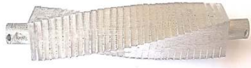
Figure 6. Chromium electroplated test part
