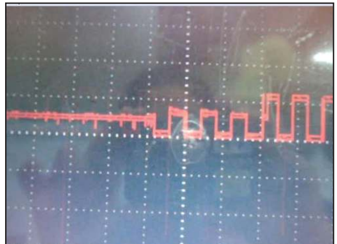
Fig. 9 DAC output for 15kV discharge on FRC
