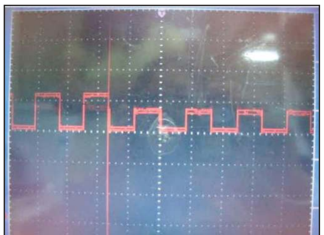
Fig. 10 DAC output when 2kV was given to pin 190
