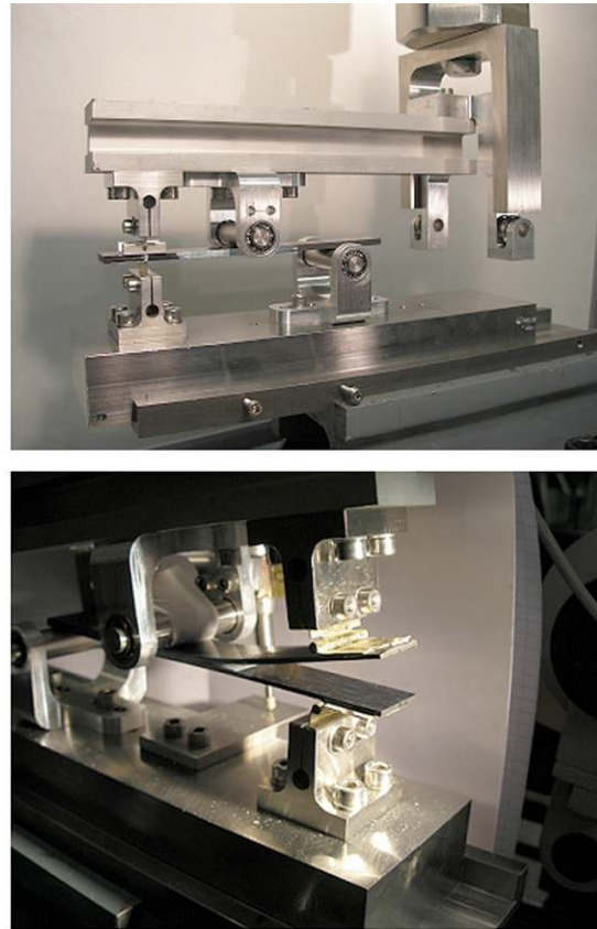
Fig. 1. Apparatus configuration and loading description of MMB test apparatus.
