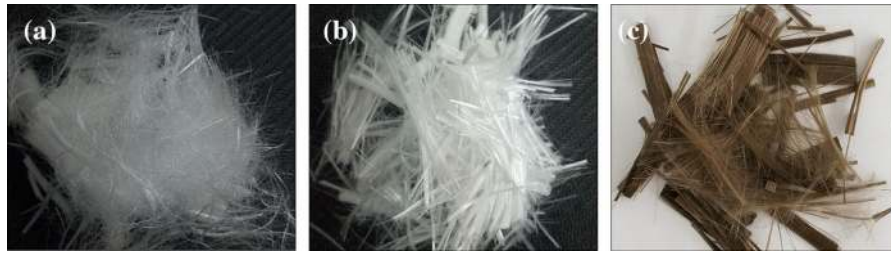
Fig. 3 a Polypropylene fibre, b Glass fibre and c Basalt fibre
