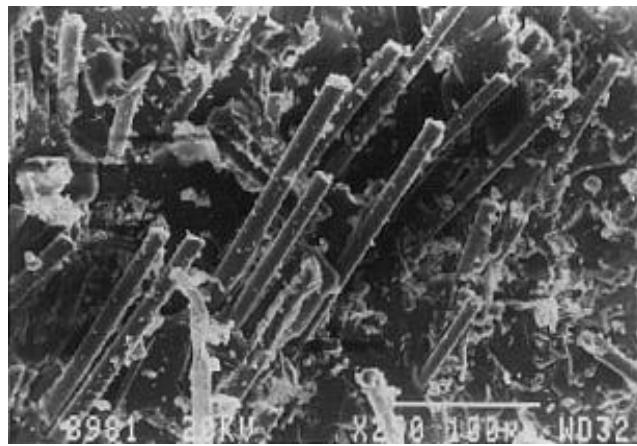
Figure 5. Fibre pull-out on the surface of impact tested specimens.
