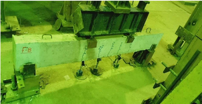
Fig. 18: During 1/3 loaded – before fire for the beam (F-B).
