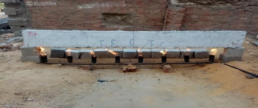
Fig. 16: During the fire for the beam (F-S).
