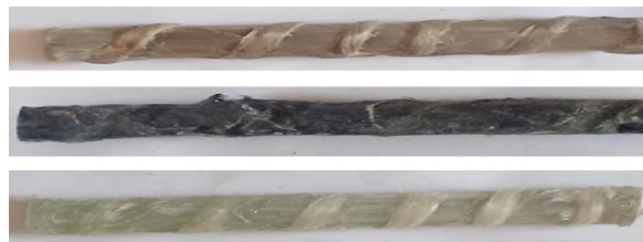
Fig. 2: BFRP & GFRP and CFRP shape after production.
