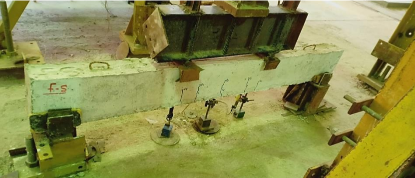
Fig. 15: During 1/3 loaded – before fire for the beam (F-S).
