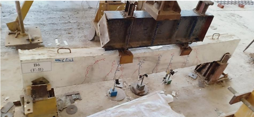
Fig. 20: After the fire and loading at failure load for the beam (F-B).
