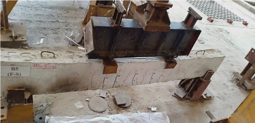
Fig. 17: After the fire and loading at failure load for the beam (F-S).
