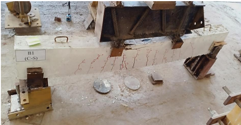
Fig. 9: Cracks pattern and failure mode of the beam (C-S).
