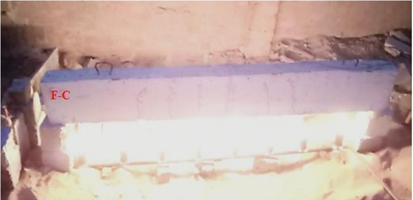
Fig. 22: During the fire for the beam (F-C).
