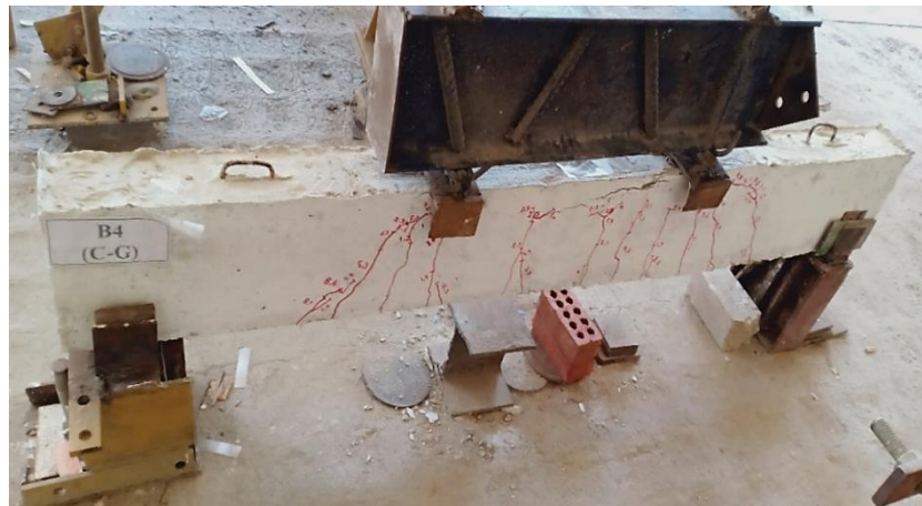
Fig. 12: Cracks pattern and failure mode of the beam (C-G).
