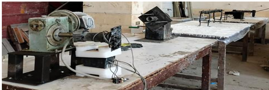
Fig. 1: The equipment used in the production of fiber bars (stand & resin bath & guide & die & motor and equipment for the production of rough bar surface).
