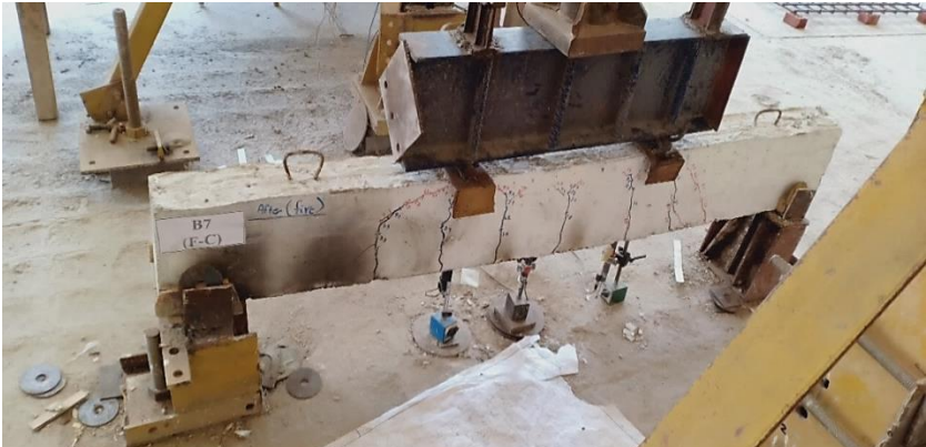
Fig. 23: After the fire and loading at failure load for the beam (F-C).
