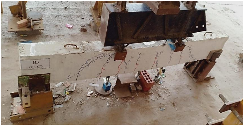
Fig. 11: Cracks pattern and failure mode of the beam (C-C).
