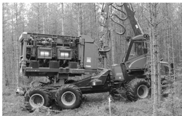
Fig. 1 The bundle-harvester system
