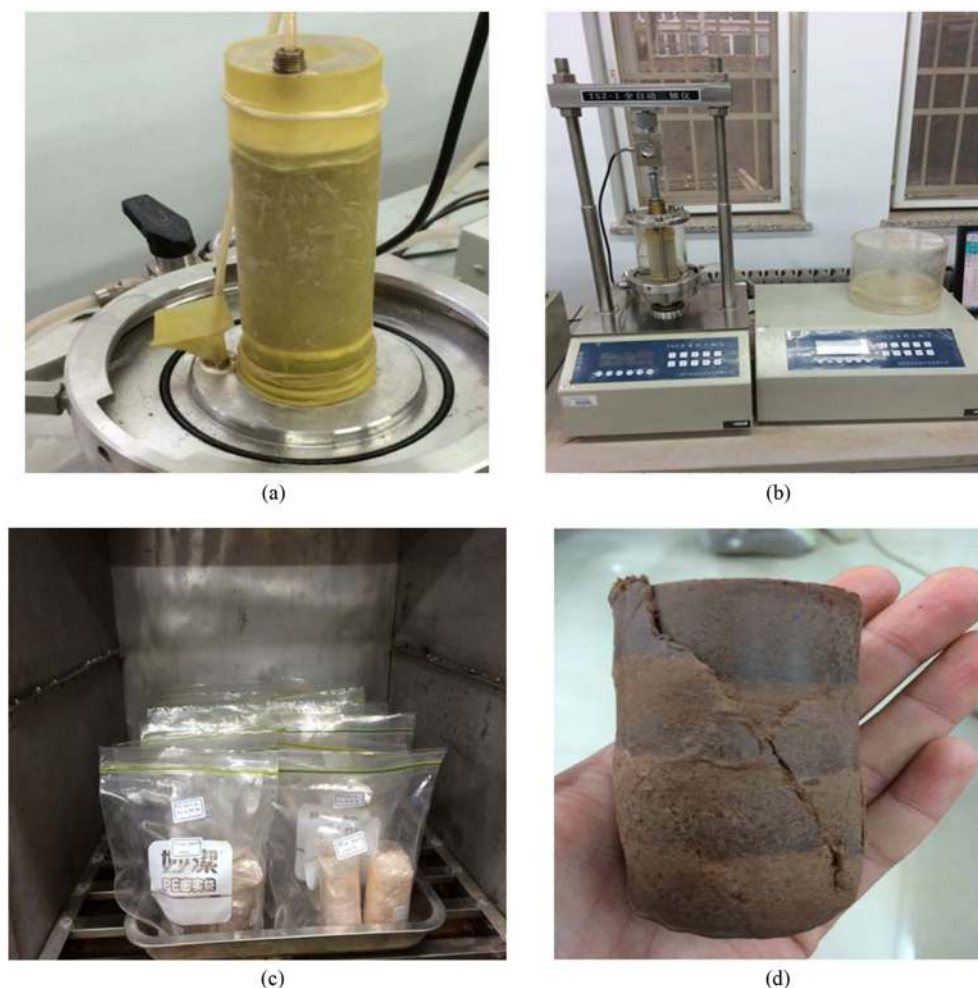
Fig. 3. Preparation of Soil Specimens for Triaxial Testing: (a) The Specimen Covered Membrane before Tests, (b) The Triaxial Compression Test System, (c) The Freeze-thaw Cabinet, (d) The Specimen after Tests
