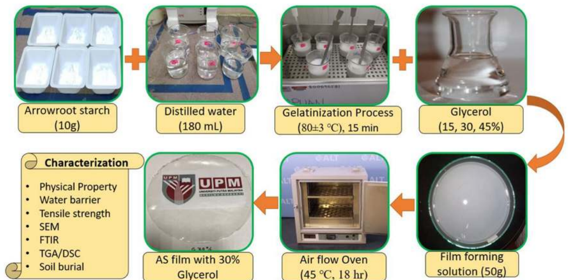
Figure 1. Flow diagram of film making process (Solution casting method).
