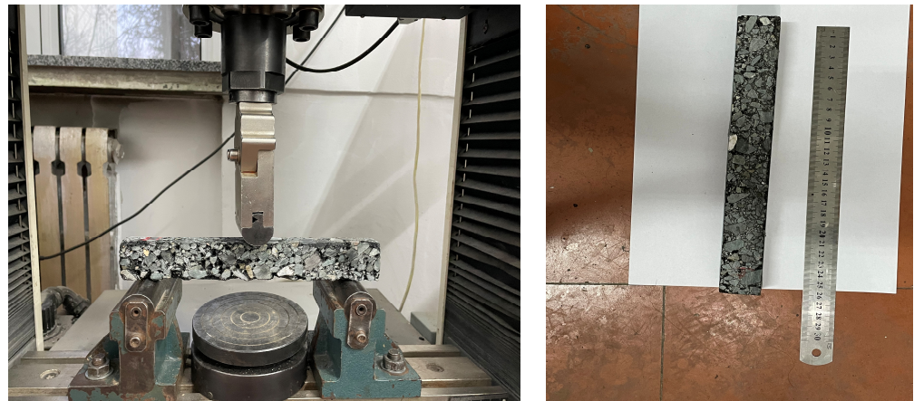
Figure 4. Process diagram of the low-temperature bending test for small beams.
