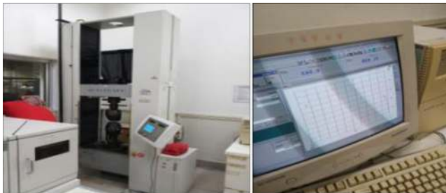
Figure 10. Tensile testing setup: CNC machine model Shimadzu/AG-G-250KN.
