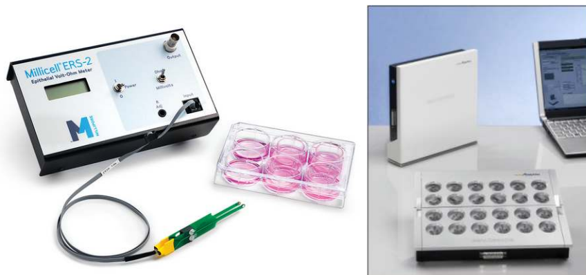
Figure 3.3: Instruments used to determine trans-epithelial resistance. On the left the Millicell ERS-2 Volt-Ohm Meter [156] on the right the cellZscope® from nano Analytics [157]
