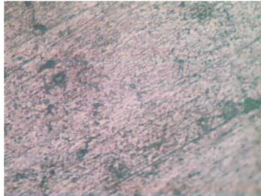
Fig. 10: Microstructure of tempered NST 37-2 steel (x400)
