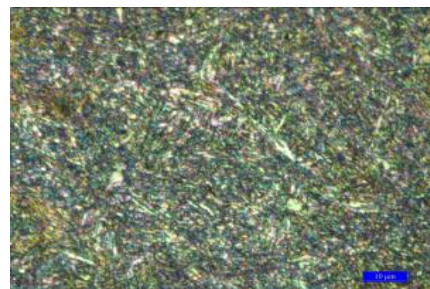
Figure 10. Oil Quench and Tempered at 500°C for 1 hr
