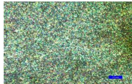
Figure 19. Oil Quench and Tempered at 550°C for 3 hr
