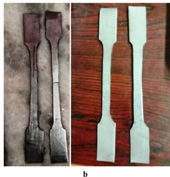
Fig. 3 a Tensile stress–strain curves at different heat treatment temperatures. b Prepared and fractured tensile test specimen
