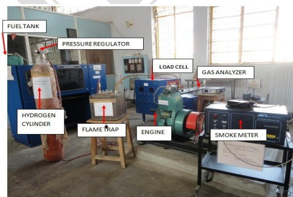
Fig.1 Photographic view of the engine experimental set up
