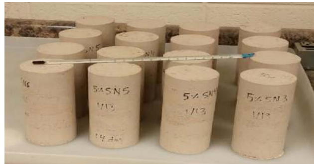
Fig. 2 UCS samples for curing in open air environment
