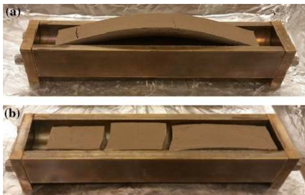
Fig. 4 a Bowing effect in Soil A, b cracking of Soil A sample
