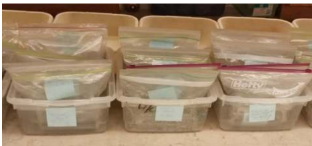
Fig. 1 UCS samples for curing in confined environment
