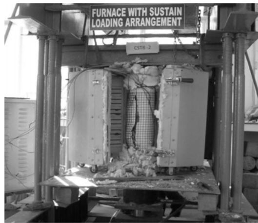
Figure 1. Set-up of furnace with sustained loading arrangement.
