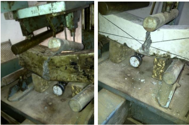
Fig. 12. specimen beam pattern collapse.
