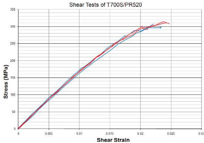
Figure 6.—Shear stress versus shear strain curves for the T700S/PR520 material system.
